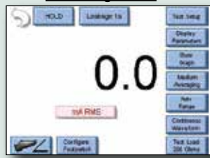
RF Leakage Mode
